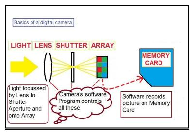
**Array of sensors:** old cameras recorded the picture on light sensitive film. Digital cameras have an **array** of light sensitive **sensors**, millions of them in a rectangular **array**. Visualise a camera taking a 5 **megapixel** picture **as**
